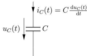
The diagram shows a capacitor symbol consisting of two parallel horizontal lines. A vertical line passes through the center of the capacitor. An arrow points downwards from the top of this vertical line, labeled with the current  $i_C(t) = C \frac{du_C(t)}{dt}$ . To the left of the capacitor, another arrow points downwards, labeled with the voltage  $u_C(t)$ .
