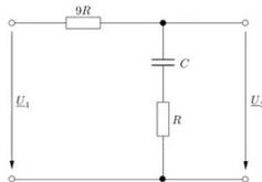
$$\underline{k} = \frac{1 + j \frac{\omega}{\omega_{g1}}}{1 + j \frac{\omega}{\omega_{g2}}}$$
