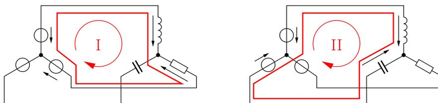
$$\begin{aligned}\underline{U}_{12} &= \underline{U}_L - \underline{U}_R, \\ \underline{U}_{31} &= \underline{U}_C - \underline{U}_L.\end{aligned}$$
